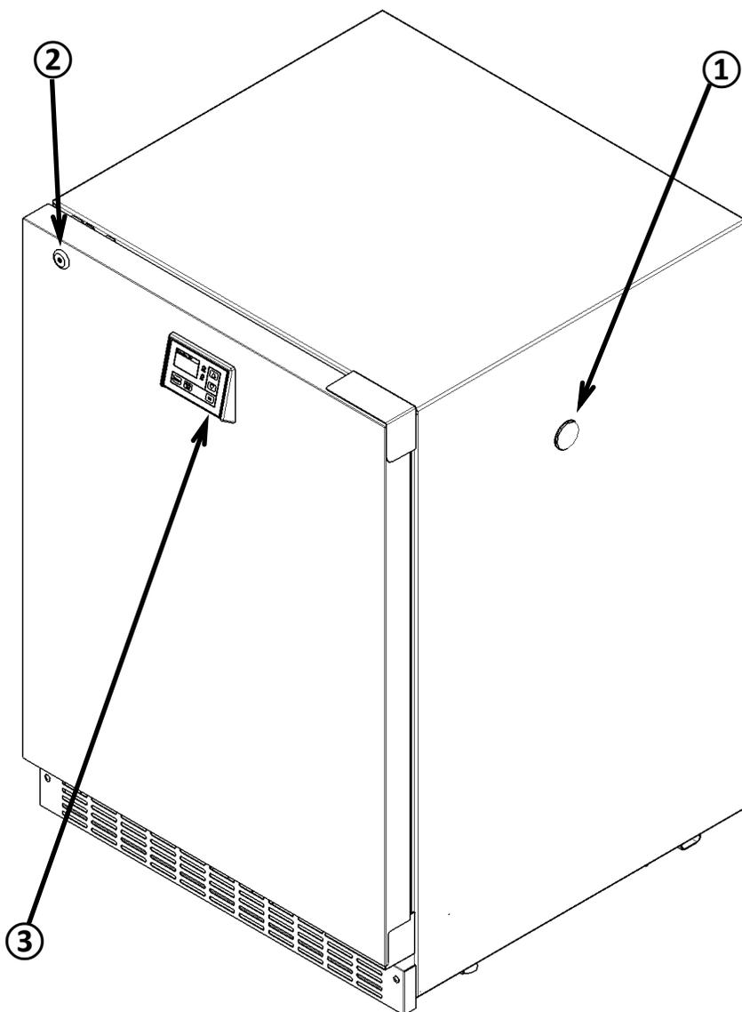
1. **Access Port:** Allow installation of temperature sensor inside the cabinet for the purpose of external monitoring.
