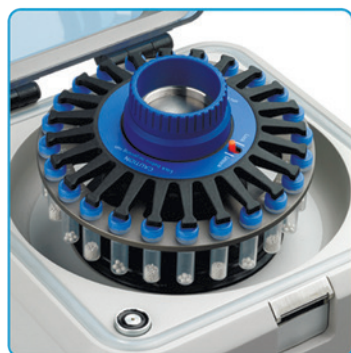
Stainless steel, 24 position tube carrier
