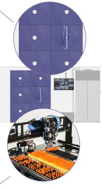
A four-lane selector allows a return order to be reformatted back into high-density storage trays and at the same time as cherry picking an order for output on the same picker. This will reduce order processing time and improve the efficiency of the store.
