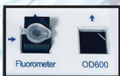
Cuvette port for OD600 and Fluorometer port
