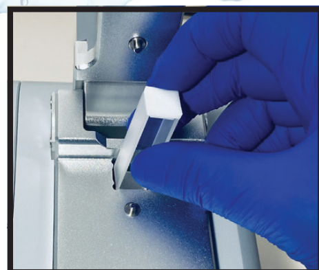
Cuvette port for OD600 readings
