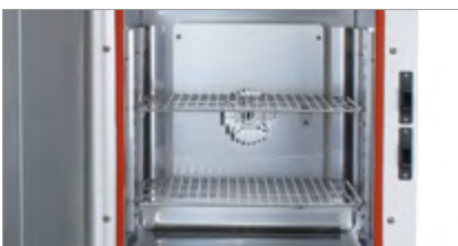
Inside of forced convection oven
