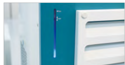
Convenient bath fluid level checking.
