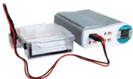
Connection to Power Supply
