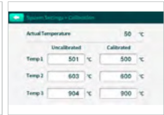
Precision temperature control with a 3-point calibration process
