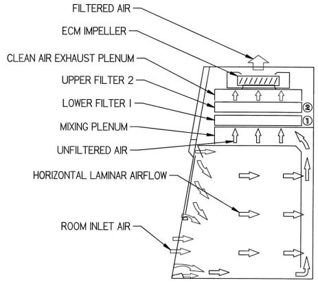
Figure 4-2 Airflow Diagram
