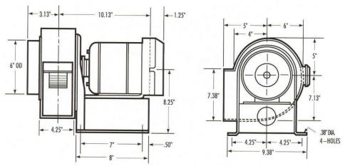
10" nominal ID inlet blower has a 1/4 hp or 1/3 hp adjustable belt drive motor and corrosion resistant epoxy coated steel housing and wheel with blower inlet of 10.87" ID. Outlet dimensions are 5.5" x 10" OD.
