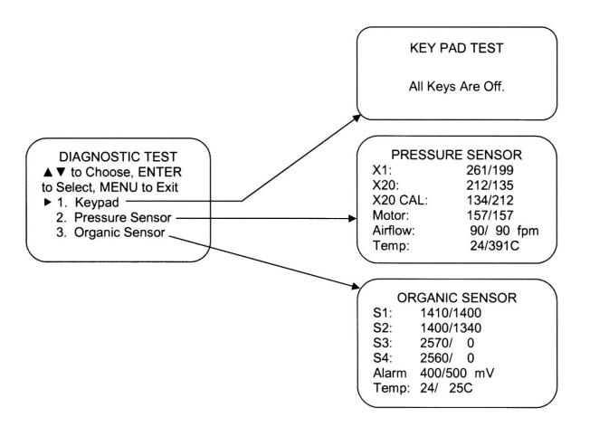
Pressure Sensor Diagnostic Notes: X20 CAL example represents a pressure of 134 with the impeller off and 212 with the motor speed at 157 producing 90 fpm for this calibration example. With Smart Flow enabled, the Paramount maintains constant pressure as indicated by the pitot tube and pressure sensor to maintain constant airflow face velocity.
