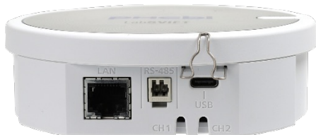
Interface ports on LabSVIFT transmitter MTR-IOTWE1-PA
