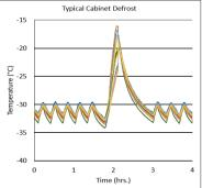
Notes an Performance Data: Performance data acquired at 22°C ambient, 5°C/-33°C naminal set points in an empty cabinet with shelves using air probes, during stabilized steady state operation and a DAQ sampling rate of one measurement every 10 seconds
