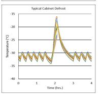
Notes on Performance Data: Performance data acquired at 22°C ambient, 5°C/-33°C nominal set points in an empty cabinet with shelves using air probes, during stabilized steady state operation and a DAQ sampling rate of one measurement every 10 seconds
