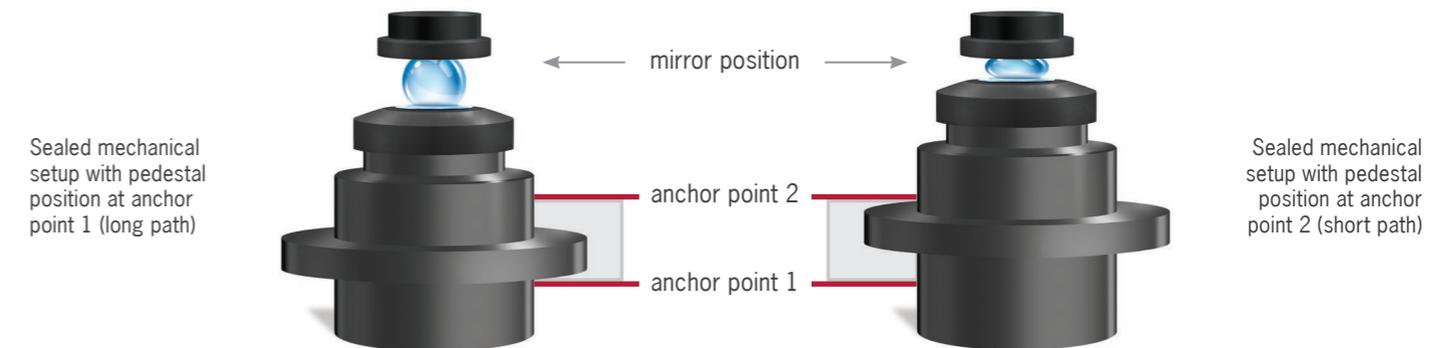
Movement between the two path lengths is controlled by a magnet. As this magnet can only position the pedestal at one of the two path lengths and cannot stop anywhere in between, path length drift is eliminated. The NanoPhotometer® is therefore recalibration-free over the lifetime of the instrument – Implen guarantees lifetime accuracy.
